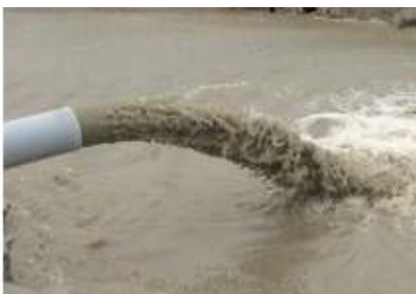
Figure 1. Beach sand slurry discharge containing 15% solids, 85% water in Japan.
